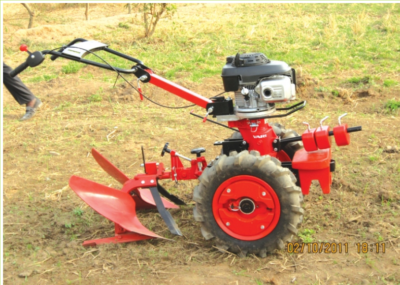
Locally manufactured machines (by NCAM in Nigeria) mounted with a PTO for bund construction, promotes mechanisation.
